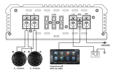
The positive and negative terminal of the subwoofer voice coil are connected to the positive and negative terminal of the amplifier
