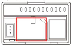
3. Insert the battery into the slot on the back of the battery cover that matches the phone's contact and battery.
