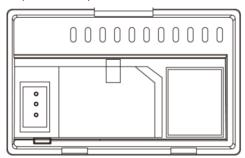
2. Insert the SIM into the device. The golden contacts on the SIM card face down and the edges align with the corresponding edges of the SIM card.
