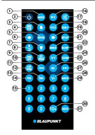
1 Press to switch between media RADIO-DISC-USB-SD-AUXIN
